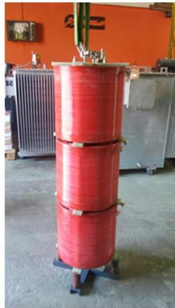
Current Limiting Reactor (PKS 10 90 400 5)
