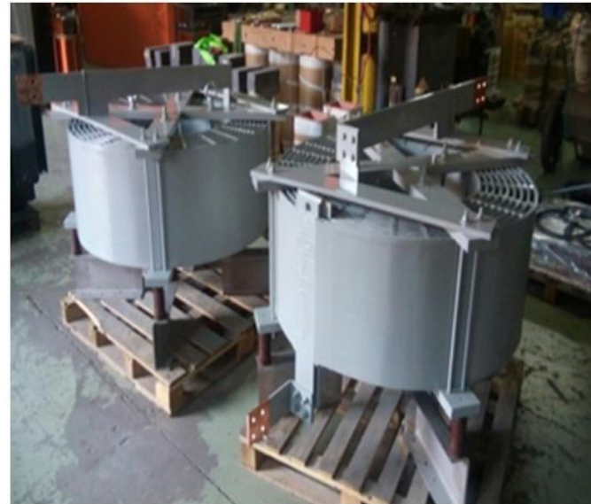
Current Limiting Reactor (PKS 2000-0,58)
